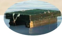
From a submerged metal platform, the cage is easily flipped over. This process is very effective at controlling fouling and secondary spat.
